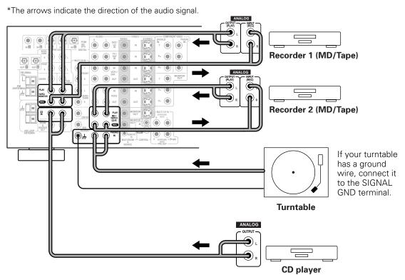
Please don't hook up any other component to the phono jacks other than a turntable. It could damage the equipment. If your turntable has a built-in amplifier please hook it up to an input other than PHONO.
